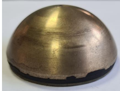
Figure 5.13 The pivot that slide on the surfaces of the FPs.
