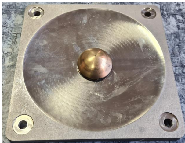
Figure 5.11 Spherical friction pendulum with radius of R=810 mm.
