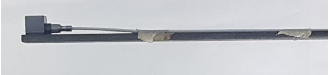
Figure 4.5. An accelerometer mounted on the test specimen
