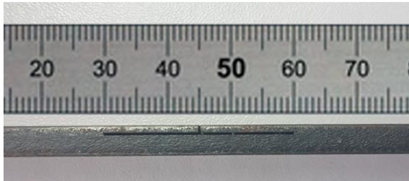
Figure 4.14. Machined T-shaped crack in Beam 2
