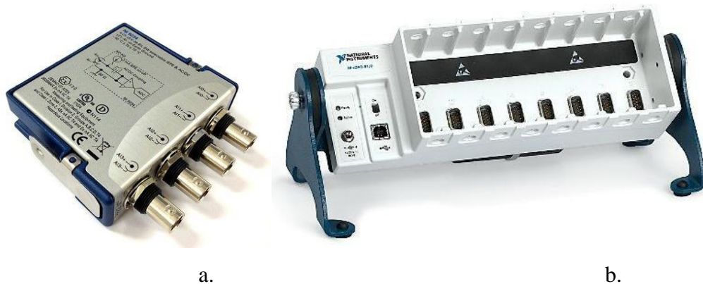
Figure 4.7. The NI 9234 acquisition module and the NI cDAQ-9172 compact chassis
