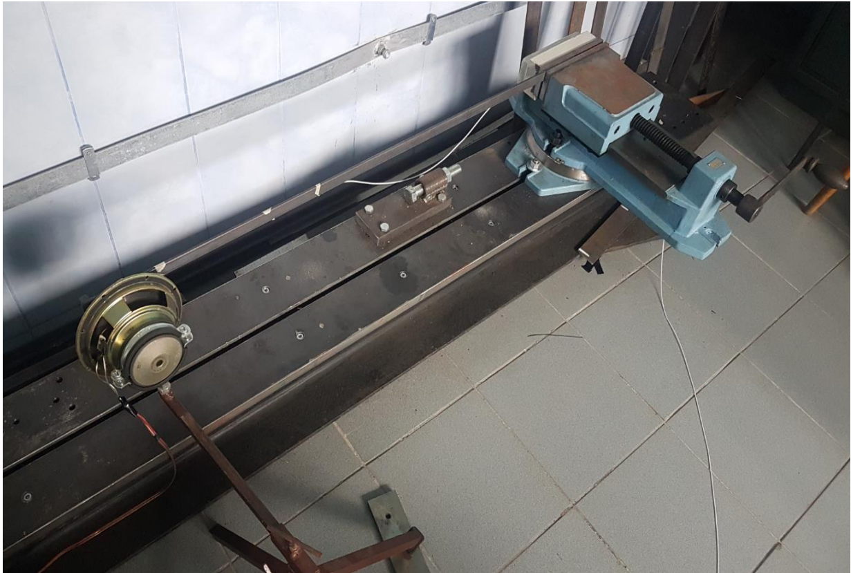
Figure 4.17. Measurement of the natural frequencies of Beam 1 on the experimental stand
